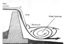
A very dangerous roller wave exists below the crest of the Princeton Dam. This roller wave can pull a boat from downstream against the toe of the dam and hold it there, rolling over and over again. It's not unusual to see logs and other debris turning in the roller wave for weeks or months.
